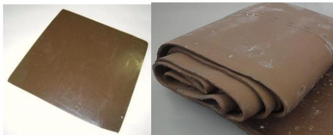
**Figure 1.** First REWASTEE multifunctional material (made of 70% EAFD).
