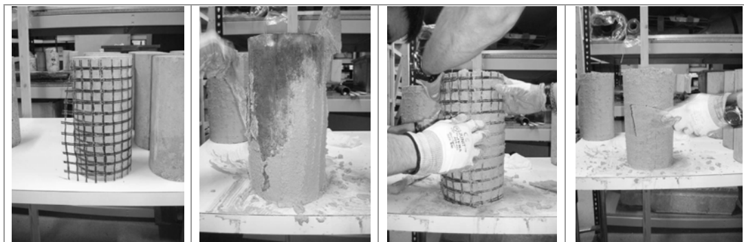
Figure 3 : Concrete confinement procedure
